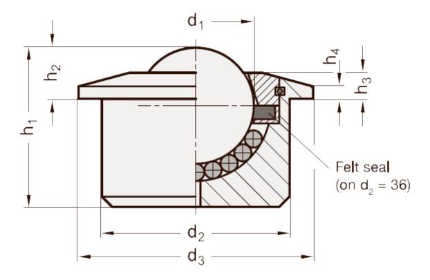
$$\begin{array}{lll} d1 & = 30.1 \\ d2 + / -0.08 & = 45 \\ d3 & = 55 \\ h1 + / -0.3 & = 36.8 \\ h2 + / -0.3 & = 13.8 \\ h3 + / -0.3 & = 7 \\ h4 & = 4.5 \\ Max load (N) = 2500 \end{array}$$
